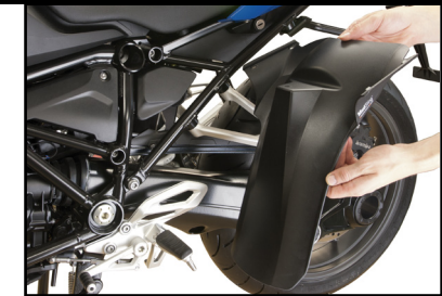
3 Hold the MudSling next to the bike in the direction of installation.
