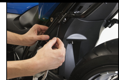
6 Install zip ties upward from the bottom through the slots, and around the frame.
