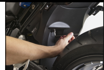
9 Using 5mm Allen Wrench, tighten the M6 Screw. You can adjust clearance between tire and swingarm with the screw, if needed. DO NOT OVERTIGHTEN.
