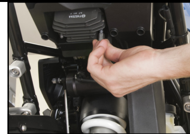
2 Apply a small amount of Loctite 248 to threaded stud. Install Coupling Hex Nut. Secure with a 10mm Open-End Wrench. DO NOT OVERTIGHTEN
